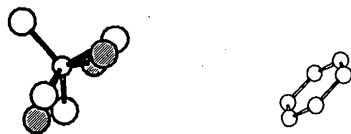
Fig. 3. Comparison of the molecular orientations of disordered CCl 4 and ordered benzene in the same crystal lattice.
